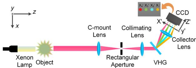
**Fig. 3** Experimental setup of the simultaneous multispectral imaging system. The multiplexed VHG is placed on the Fourier plane of the  $4f$  system combined with the collimating lens and the collector lens. Each hologram diffracts the Bragg-matched component of the incident beam. The collector lens projects laterally separated images formed with different wavelengths on the CCD camera.
