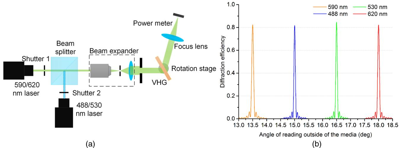
**Fig. 2** (a) Experimental setup for measuring the spectral-angular selectivity at different target wavelengths. (b) The measured spectral-angular selectivity curves of the four multiplexed volume holograms. The diffraction intensity of each laser beam is measured sequentially by switching the shutter placed in front of the laser head. The results show that the Bragg-matched diffraction efficiency of each hologram is higher than 0.8.
