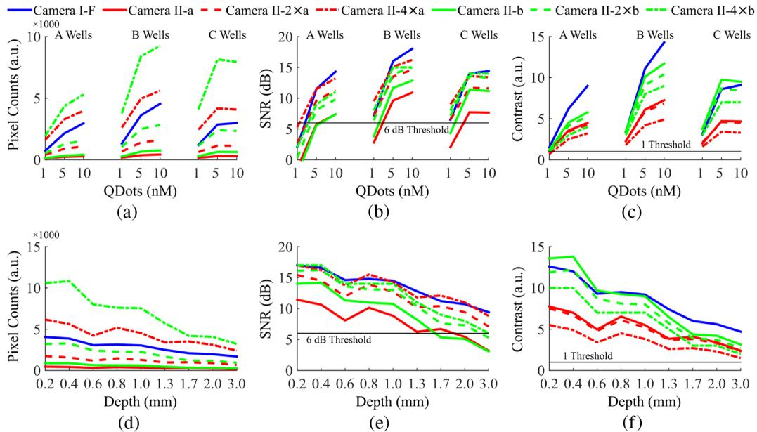
**Fig. 7** Quantitative comparisons between camera I-F and all configurations of camera II. (a) Pixel counts, (b) SNR, and (c) contrast from the nine wells with different optical properties. (d) Pixel counts, (e) SNR, and (f) contrast from the nine wells with different depths from the phantom's top surface. In all panels, x-axis labeling corresponds to the labeling of phantom elements shown in Fig. 1(b).
