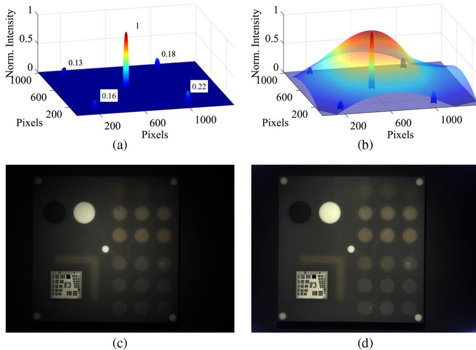
**Fig. 8** Field illumination correction through reflectance measurements. (a) The normalized intensity of the five highly scattering wells of the phantom. (b) The field illumination profile over the entire field of view. (c) An acquired image from the color camera of camera I affected by vignetting. (d) Application of flat-fielding to correct for inhomogeneous field illumination.
