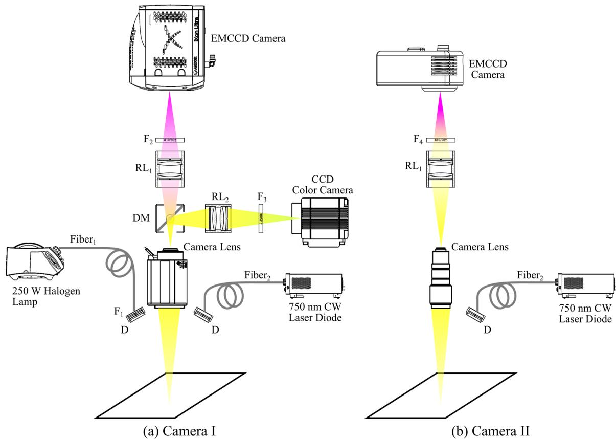
**Fig. 2** Schematics of the two imaging systems employed in this study. (a) The fluorescence/color camera (camera I) and (b) the fluorescence camera (camera II) were validated and benchmarked through imaging the composite phantom. D: diffuser; F: filter; DM: dichroic mirror; RL: relay lens.
