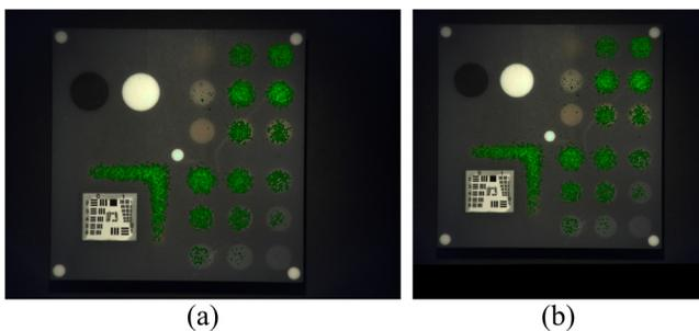
**Fig. 9** A color image of the phantom augmented with fluorescence data as acquired by camera I-FC. (a) The augmented image in its original coordinates system. (b) The augmented image transformed to the coordinates system of the fluorescence image.
