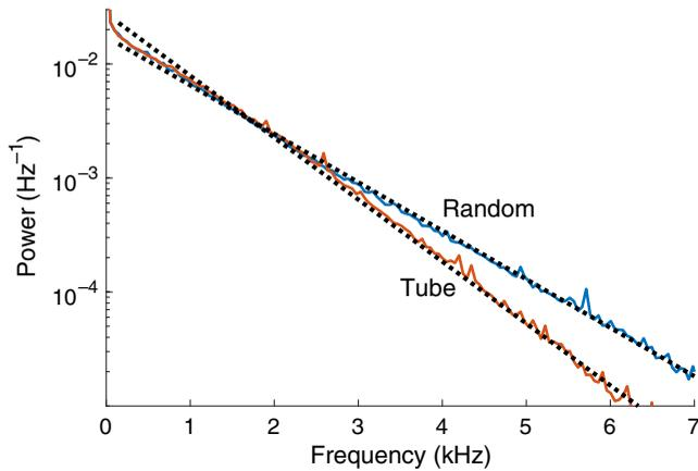
**Fig. 4** Simulated Doppler power spectrum assuming laminar flow (parabolic speed distribution), with the RBC velocity vectors in the tube direction (red) or random direction (blue). Dotted lines show fitted exponential decay functions.
