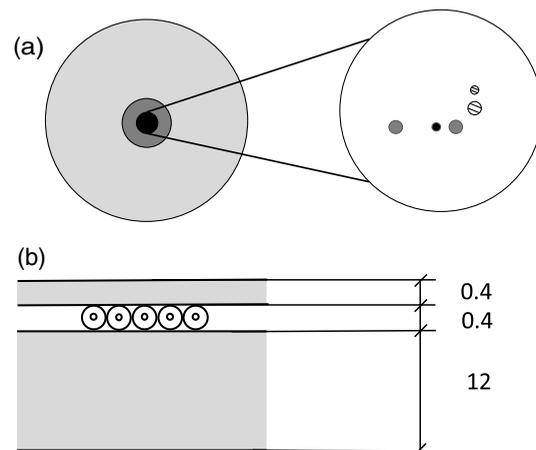
**Fig. 2** (a) Face of the probe with source–detector geometry. The central black region with fibers includes two LDF fibers,  $D = 125 \mu\text{m}$  (striped: emitting, black: detecting) and three DRS fibers,  $D = 200 \mu\text{m}$  (striped: emitting, gray: detecting). (b) Schematic view of the flow phantom. Gray structures are made of silicone and the gap between the silicone slabs and the tubes are filled with ultrasound gel. Measurements are in millimeter.
