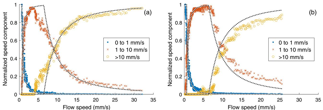
**Fig. 5** Normalized speed components versus the flow speed in the tube for (a) measurement 1 and (b) measurement 2. The dotted lines mark the theoretically expected speed component assuming a laminar flow in the tube direction.
