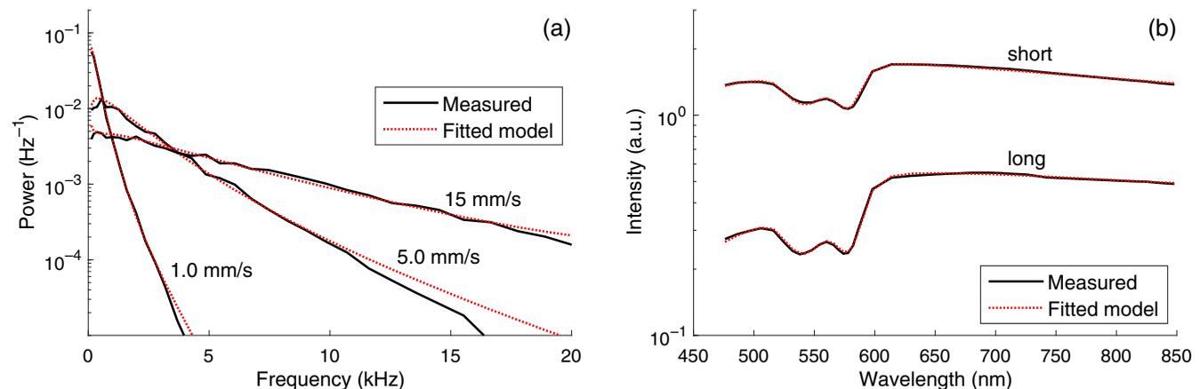
**Fig. 3** (a) Three examples from measurement 1 of measured (solid) and fitted (dotted) LDF spectrum covering the range from 1.0 to 15 mm/s. (b) Example of measured (solid) and fitted (dotted) DRS spectrum for the short- and long-fiber separation in the EPOS system, taken at the same time point as the 5.0 mm/s LDF spectrum example. The fitting error was within 3% for both separations and without any systematic deviations.
