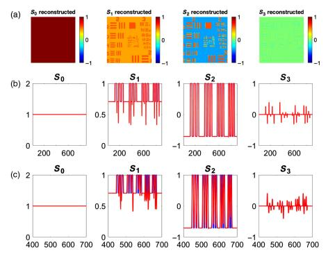
**Fig. 8** Stokes vector of a USAF target reconstructed with the sliding reconstruction method (a) showing traces of the (b) largest and (c) smallest blocks of resolution dashes. As can be observed from the changes from the raw signal to the reconstructed signal, strong discontinuities create artifacts in the Stokes images.
