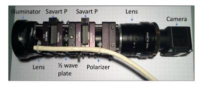
Fig. 3 The snapshot Mueller matrix polarimeter.
