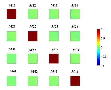
**Fig. 9** Mueller matrix of air. The portable device was tested in transmission to understand the error of the polarimetric response. Although some structural artifacts are present (small white lines in the matrix), the expected values of ones in main diagonal elements are present.
