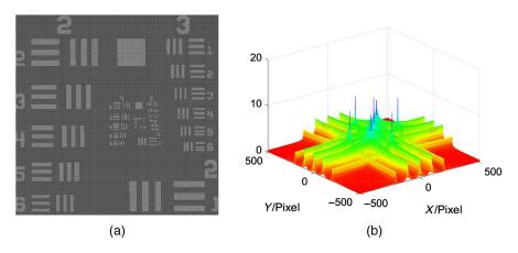
**Fig. 6** (a) Interferogram associated with the USAF test target as seen by a camera sensor, (b) Fourier transform of the interferogram of the USAF target, featuring the peaks (along with the full frequency profile) where the Stokes vectors are spatially encoded within the interferogram.
