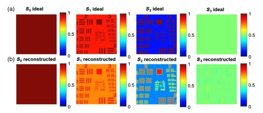
**Fig. 5** (a) An input Stokes vector was created with a USAF target. The status of polarization corresponds to a linear orientation of 22.5 deg for the background and 0 deg for the lines. (b) The Stokes vector after reconstruction. There are still visible artifacts (traces from the target) where the Fourier reconstruction failed.
