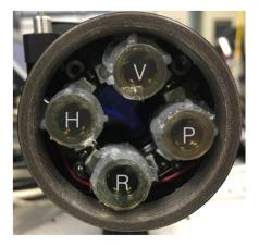
**Fig. 4** Polarization state generator. H is a horizontally aligned polarizer (with respect to the reference frame, optical bench), V is a vertically aligned polarizer, P is a 45 deg aligned polarizer, and R is a circular polarizer.
