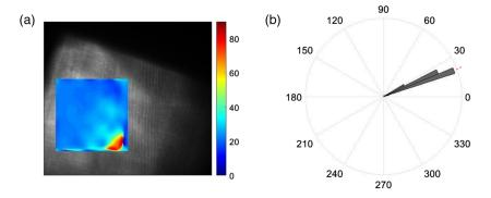
**Fig. 10** Extruded silicone sample recovered orientation. The silicone sample was placed at a 22-deg shift (marked in the red line) from the frame of reference. (a) Raw image (gray scale) with the recovered mean angle of a region of interest (colormap) and (b) circular histogram of the recovered angles.
