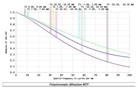
Fig. 2 MTF of the Savart polarimeter.
