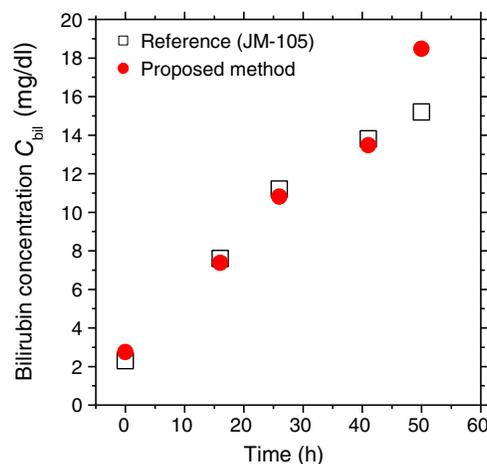
**Fig. 6** Typical time courses of transcutaneous bilirubin concentration  $C_{bil}$  estimated from the diffuse reflectance spectra measured by the spectrometer and those measured by a commercially available bilirubinometer before and after bile duct ligation.
