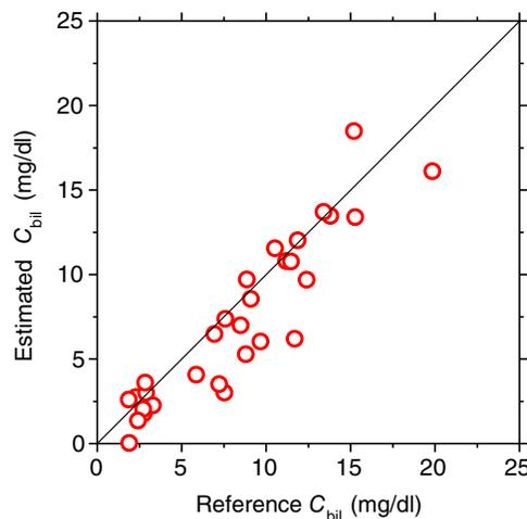
**Fig. 8** Comparison between the bilirubin concentration  $C_{bil}$  estimated by the proposed method and that measured by the commercially available bilirubinometer, obtained from seven samples during bile duct ligation.
