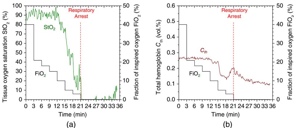
**Fig. 10** Typical time courses of (a) tissue oxygen saturation  $StO_2$  and (b) total hemoglobin concentration  $C_{th}$  obtained from the proposed method while changing  $FiO_2$ .
