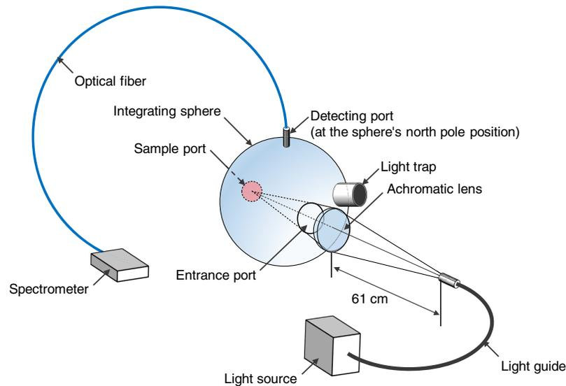
**Fig. 4** Schematic illustration of experimental setup for measuring diffuse reflectance spectra of rat dorsal skin.
