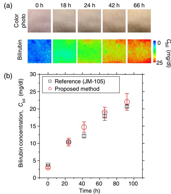
**Fig. 7** (a) Typical sequential images of  $C_{bil}$  obtained from the spectral diffuse reflectance images acquired by the hyperspectral camera before and after bile duct ligation. (b) The average value of  $C_{bil}$  over the entire region of the images shown in panel (a).
