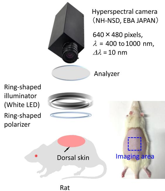
**Fig. 5** Schematic illustration of the hyperspectral diffuse reflectance imaging system.
