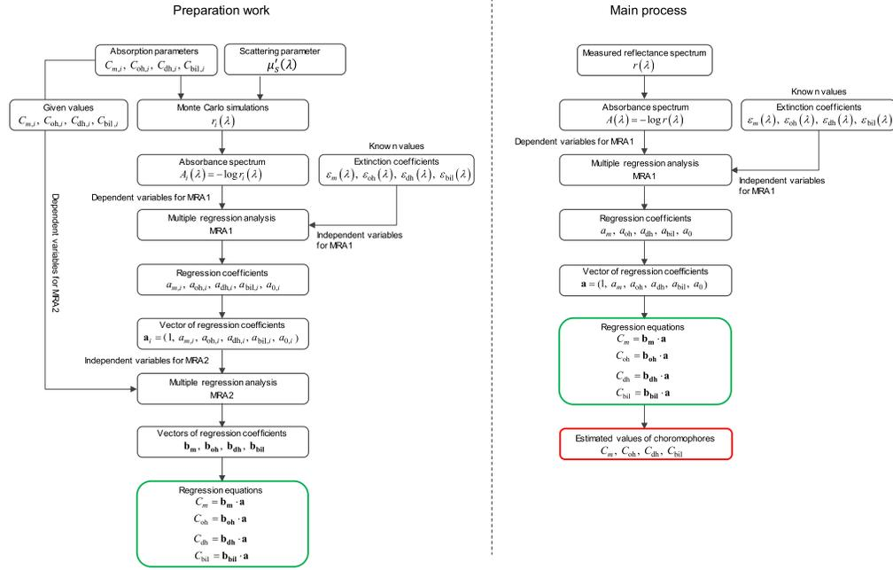
**Fig. 1** Flowchart of the process for estimating the concentrations of melanin  $C_m$ , oxygenated hemoglobin  $C_{oh}$ , deoxygenated hemoglobin  $C_{dh}$ , and bilirubin  $C_{bil}$ . (a) Preparation work for determining the regression equations and (b) main process for deriving  $C_m$ ,  $C_{oh}$ ,  $C_{dh}$ , and  $C_{bil}$  from the measured reflectance spectra.
