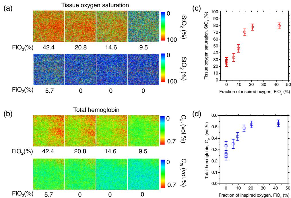
**Fig. 11** Typical sequential images of (a) tissue oxygen saturation  $StO_2$  and (b) total hemoglobin concentration  $C_{th}$  estimated from the spectral diffuse reflectance image acquired by the hyperspectral camera while changing  $FiO_2$ . The average values of  $StO_2$  and  $C_{th}$  over the entire region of each image shown in (a) and (b) are plotted in (c) and (d), respectively.
