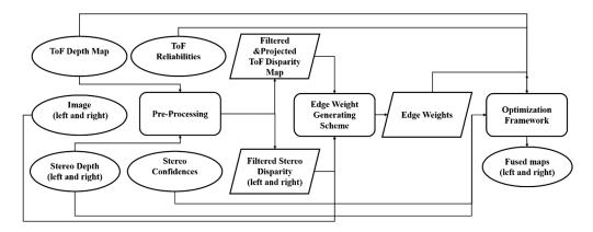
Fig. 2 An overview of the entire processing pipeline.
