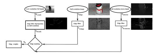
**Fig. 1** Scheme showing the generation process for the edge-weighting map  $W_E$ . The edge maps correspond to each source and are calculated with different thresholds. The edge maps exhibited here are in a horizontal direction only.
