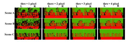
**Fig. 6** Color-coded consistency map between the right- and left-fusion maps for three scenes. Each column corresponds to a specific threshold.
