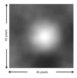
Fig. 2 Example of a test statistic map. After cropped EROC template of one specific signal scanned on all possible locations of a signal on a testing image, a statistic map associated to this testing signal is generated. The highest pixel value (brightest spot) in this map indicates the estimated location of the testing signal.
