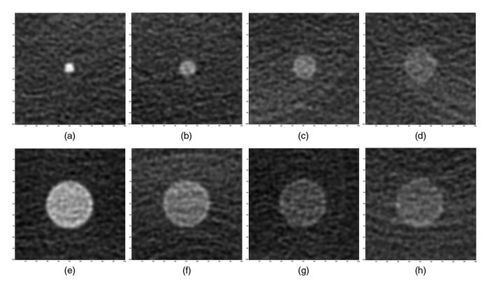
**Fig. 3** Examples of images used for combination of detection, size and contrast estimation task. All of the images shown are the averaged results of 500 FBP images. The various signal parameters are: (a) 3 mm 14 HU, (b) 5 mm 7 HU, (c) 7 mm 5 HU, (d) 10 mm 3 HU, (e) 15 mm 14 HU, (f) 15 mm 7 HU, (g) 15 mm 5 HU, and (h) 15 mm 3 HU.
