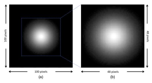
**Fig. 1** Templates: (a) original EROC template and (b) cropped EROC template. The cropped EROC template is used for scanning on the spatial domain for signal-location-unknown tasks.
