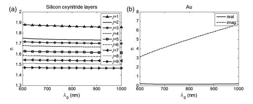
**Fig. 2** (a) Spectrums of the refractive indices of the nine silicon-oxynitride layers in each period of the 1-D PC. The imaginary parts of the refractive indices were on the order of  $10^{-4}$  (Ref. 22) and were therefore ignored. (b) Spectrums of the real and imaginary parts of the refractive index of gold.
