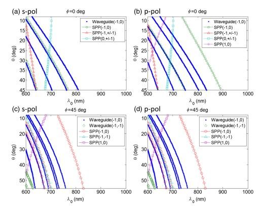
**Fig. 6** Predicted values of  $\theta$  obtained from Eq. (3) and Figs. 4 and 5 for the experimental excitation of SPP waves and waveguide modes of (a,c) s-polarization state and (b,d) p-polarization state for (a,b)  $\phi = 0$  deg and (c,d)  $\phi = 45$  deg.
