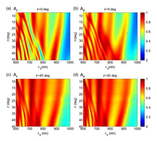
**Fig. 7** Absorptances (a,c)  $A_s$  and (b,d)  $A_p$  of the fabricated structure measured as functions of  $\lambda_0$  and  $\theta$  for (a,b)  $\phi=0$  deg and (c,d)  $\phi=45$  deg.
