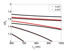
**Fig. 5** The normalized wavenumbers  $q/k_0$  of waveguide modes calculated using the transfermatrix approach.
