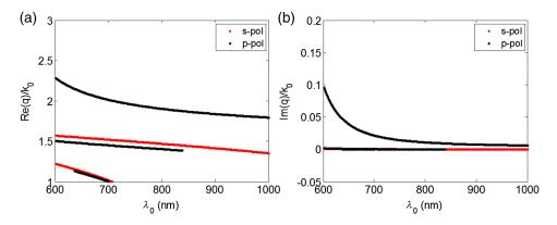
**Fig. 4** (a) Real and (b) imaginary parts of the normalized wavenumbers  $q/k_0$  of surface-plasmon-polariton (SPP) waves obtained after solving the canonical boundary-value problem.
