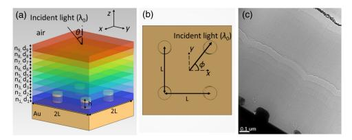
**Fig. 1** (a) Schematic of a one-dimensional (1-D) photonic crystal (PC) deposited on top of a two-dimensional (2-D) metal grating. Only one period of the PC is shown. The wavevector of the incident light is inclined at  $\theta$  with respect to the z axis, and (b) at  $\phi$  with respect to the x axis in the xy plane. (c) Transmission electron microscopy image of the fabricated sample with two periods of PC.
