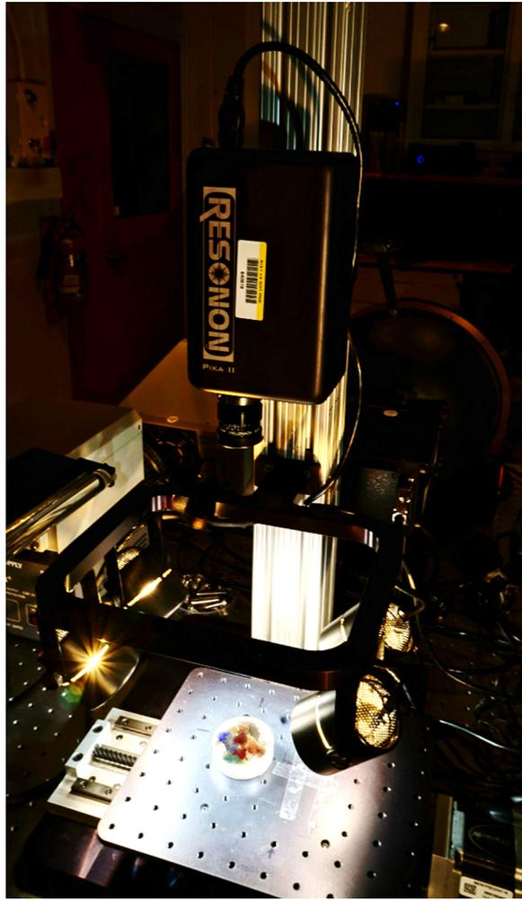
**Fig. 2** Photograph of the VNIR section of the HSI microscope. The Resonon Pika II is shown with the Xenoplan 1.4/23-0902 objective lens.
