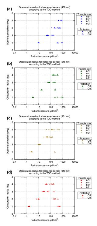
Fig. 12 Results of the TOD method for the hardened sensor: laser wavelength (a) 488 nm, (b) 515 nm, (c) 561 nm, and (d) 640 nm.
