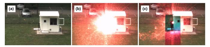
**Fig. 8** Images taken at a field trial with the hardened sensor: (a) scene without disturbing laser radiation, (b) scene with laser dazzle; the protection measure (DMD) was not activated, (c) scene with laser dazzle; the protection measure (DMD) was activated.
