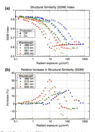
Fig. 14 Results of the SSIM analysis for the hardened sensor: (a) value of the SSIM index for the protected and unprotected case and (b) increase of the SSIM index (in percent) when the protection measure (DMD) is activated compared to the unprotected case.
