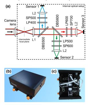
**Fig. 3** (a) Schematic diagram of the optical layout of the three-bandsensor. (b) and (c) Photographs of the three-band-sensor (without external camera lens).
