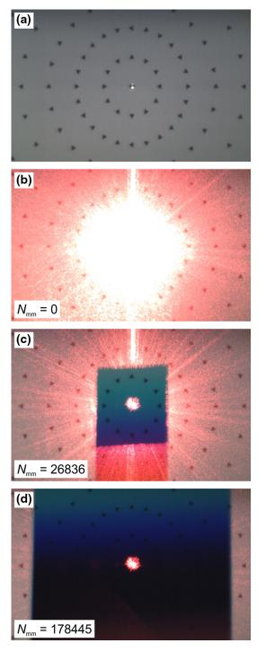
Fig. 2 Images taken with the hardened sensor (a) without and (b–d) with laser dazzle (laser wavelength  $\lambda = 640$  nm, radiant exposure  $H = 7.5 \ \mu J/cm^2$ ). The numbers of activated micromirror elements  $N_{\rm mm}$  are indicated.
