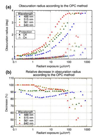
Fig. 11 Results of the OPC method for the hardened sensor: (a) obscuration radius (in degrees) according to the OPC method for the protected and unprotected case. (b) Relative decrease of the obscuration radius (in percent) when the protection measure (DMD) is activated referred to the unprotected case.
