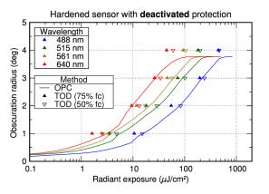
Fig. 19 Comparison of obscuration radii derived with two different data analysis methods (OPC and TOD). In the case of the TOD method, two different levels of fraction correct (75% and 50%) were used to derive the values.
