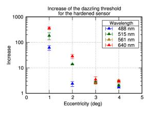
Fig. 13 Increase of the dazzling threshold for the hardened sensor when the protection measure (DMD) is switched on as a function of the eccentricity. The results for different laser wavelengths are distinguished by the color of the data points.
