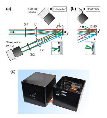
Fig. 1 Concept for hardening a sensor against laser dazzling using a DMD: (a) operation mode for regular imaging, (b) operation mode with high attenuation of dazzling laser light, and (c) photograph of the hardened sensor.
