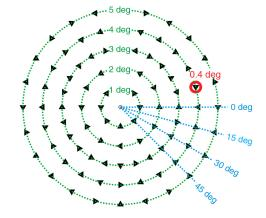
**Fig. 7** Sketch of a test chart used for the laboratory experiments (triangle size 0.4 deg). Triangles of one size with different orientation are aligned on five concentric circles with eccentricities ranging from 1 to 5 deg. For each triangle size (diameter of the circumscribed circle ranging from 0.1 to 0.5 deg), a separate test chart was prepared.
