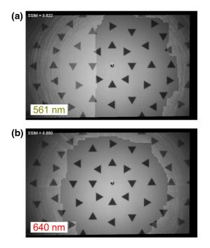
Fig. 18 Images taken with the three-band-sensor for the radiant exposures levels where the lowest value of SSIM index occurred. (a) Laser wavelength 561 nm and (b) 640 nm.
