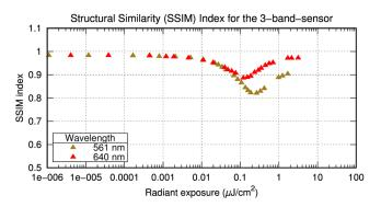
Fig. 17 Results of the SSIM analysis for the three-band-sensor.
