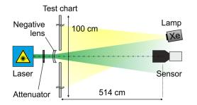
Fig. 6 Sketch of the experimental setup for quantitative evaluation of laser dazzling.
