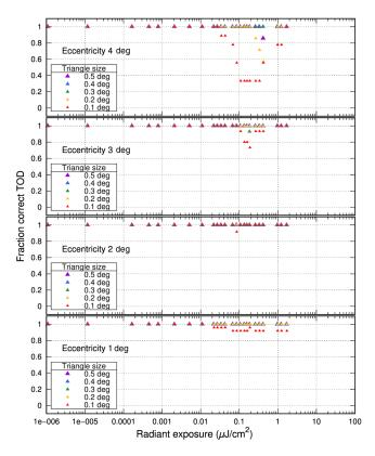
**Fig. 16** Fraction correct (laser wavelength  $\lambda = 561$  nm) as a function of radiant exposure for the three-band-sensor.
