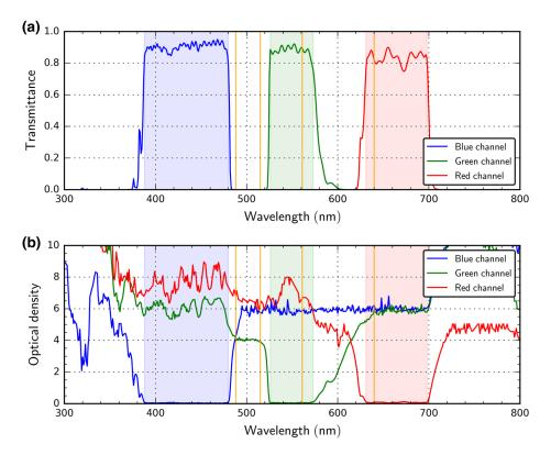
Fig. 5 Calculated optical properties of the three-band-sensor: (a) transmittance and (b) optical density as a function of wavelength. The laser wavelengths used for the laboratory measurements are marked by orange colored, vertical lines. The passbands of the three channels are highlighted by colored background.
