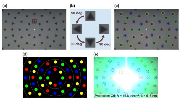
**Fig. 9** Image analysis by means of TOD: (a) an undazzled image is used to extract a template (orientation: up), (b) all other orientations (left, down, right) are generated by rotating the extracted template, (c) template matching is performed on an undazzled image to produce (d) a map of the triangle existing in the scene. (e) Example of template matching that is performed on a dazzled image.
