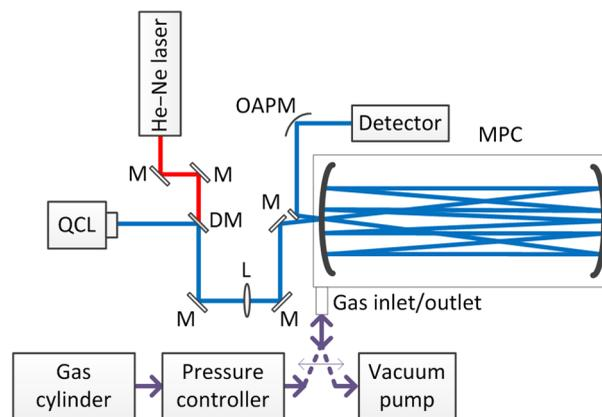
**Fig. 2** Schematic diagram of the setup. M, mirror; DM, dichroic mirror; OAPM, off-axis parabolic mirror; L, lens (500-mm focal length); and MPC, multipass cell. He-Ne laser was used for system alignment.
