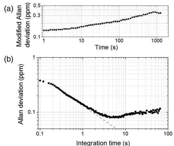
**Fig. 5** (b) Allan deviation and (a) modified, two-point Allan deviation measured when laser wavelength was adjusted to target center of H<sub>2</sub>S transition.
