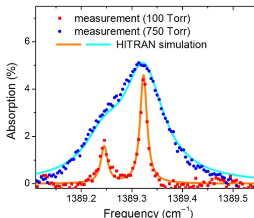
**Fig. 3**  $\text{H}_2\text{S}$  spectra recorded for pressures of 100 and 750 Torr (sample is 200 ppmv of  $\text{H}_2\text{S}$  balanced in nitrogen, 76-m path length). In both cases, good agreement with HITRAN-based simulation is obtained.
