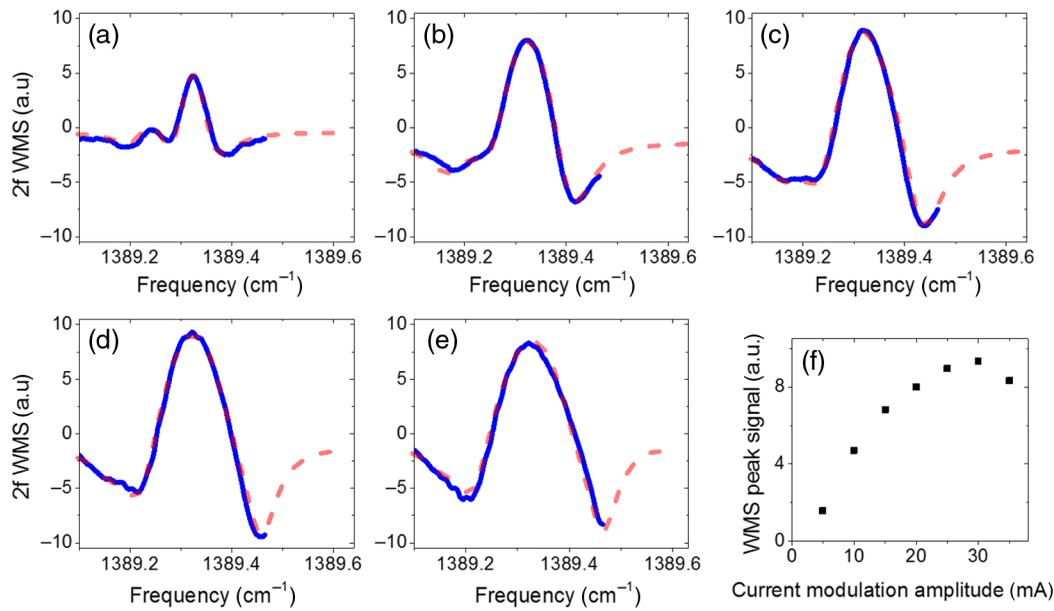
**Fig. 4** (a)–(e) 2f WMS spectra recorded for different amplitudes of current modulation (5, 15, 25, 30, and 35 mA). Blue solid line, measured signal; dashed red line, HITRAN-based simulation (for large modulation amplitudes part of the spectrum was not recorded due to limited tuning range of the source); (f) 2f WMS amplitude at the transition center plotted in function of current modulation amplitude.
