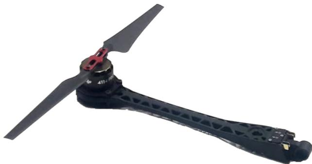
Fig. 1 DJI S800 EVO propulsion system.
