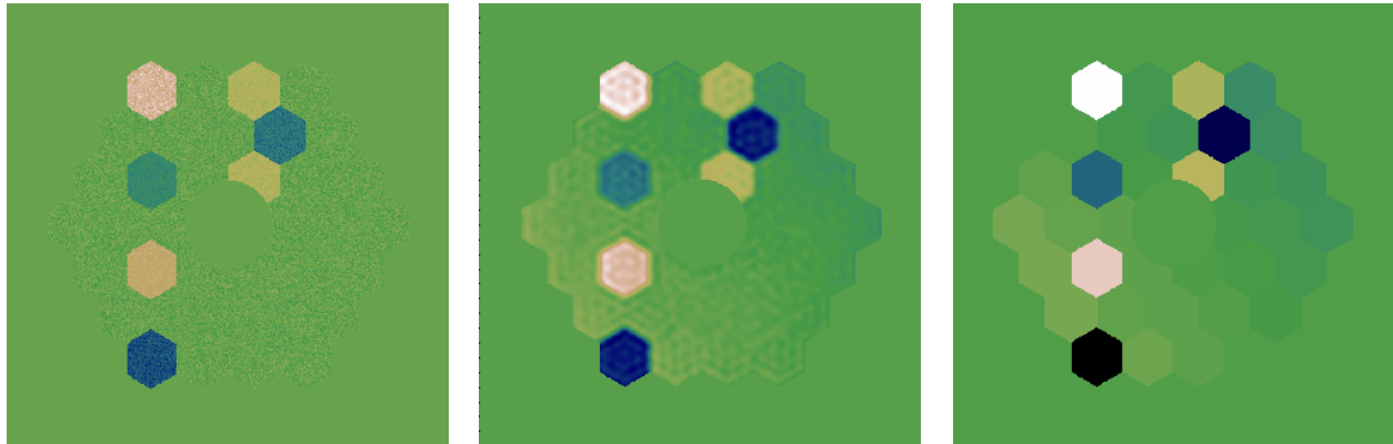
Figure 10: Left: Input phase map. Middle: Retrieved phase map. Right: Projected segment piston error.
