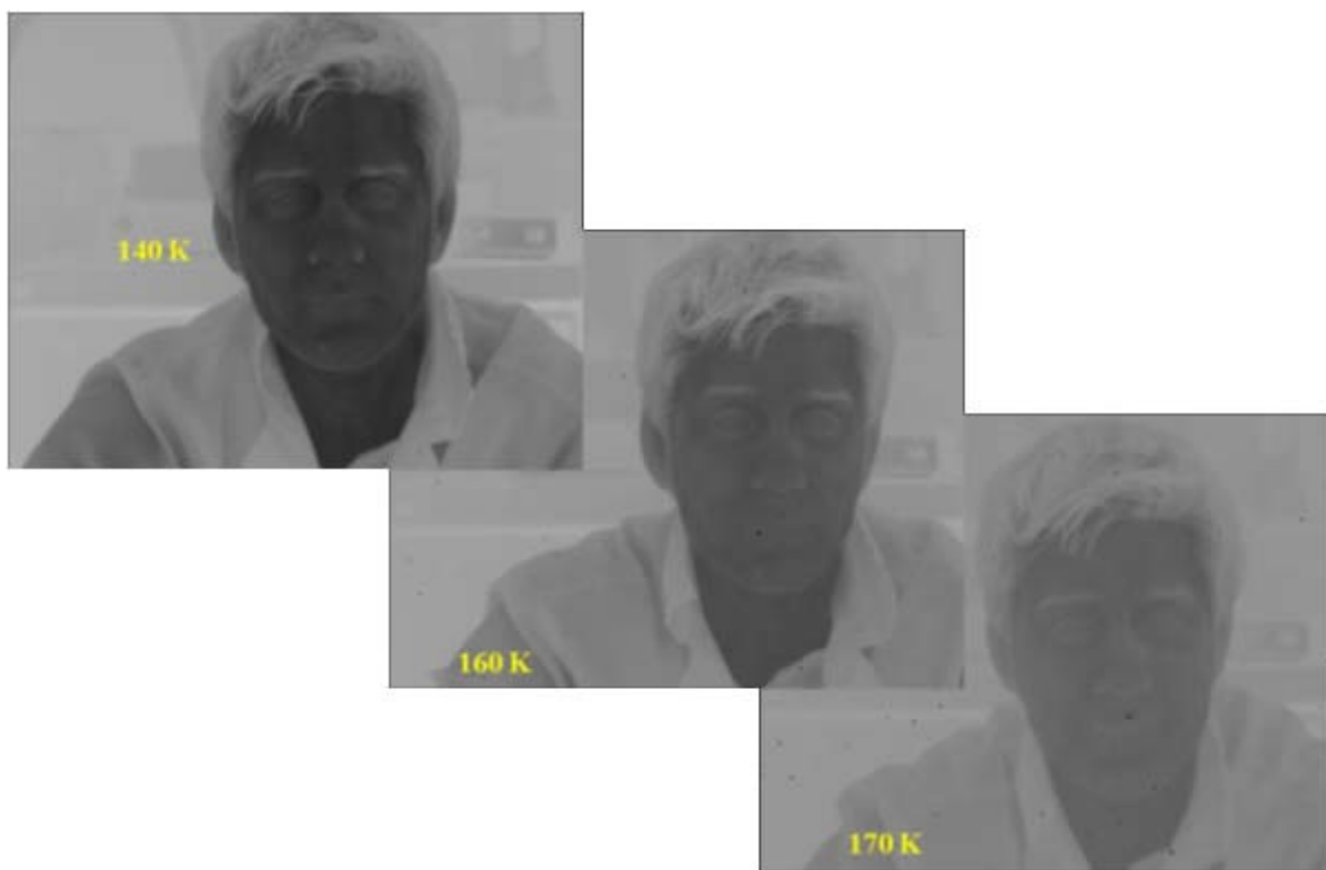
Fig. 8. Infrared images taken with an F/3.5 optics at FPA temperatures of 140, 160, and 170 K with a HOT detector fabricated in the most recent technology (end of 2013). The detector has a 640x512 pixel format with 15 \mu\text{m} pitch and a cut-off wavelength of 4.75 \mu\text{m} at 160 K.
