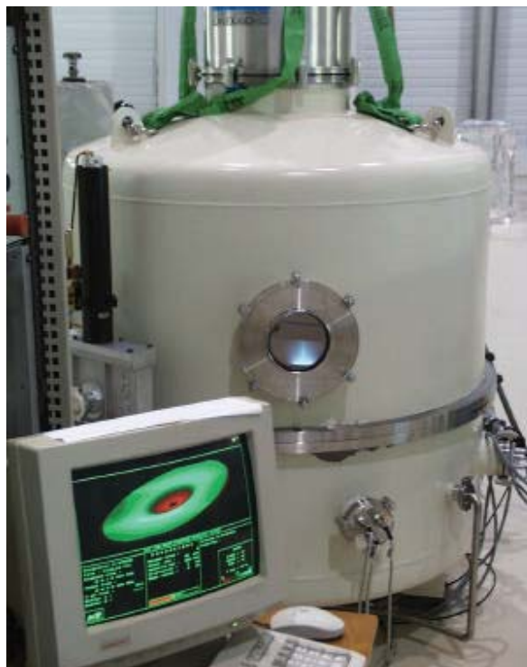
Fig. 1. The vacuum chamber of the IBF facility during the correction of a mirror. The ion beam can be seen through the window.
