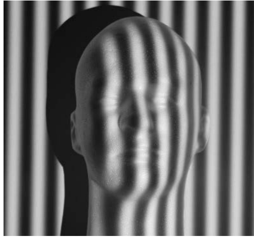
Figure 2. An example of the deformed fringe pattern from a manikin head target. Notice the shadow that does not have any fringe information, which can lead to erroneous phase unwrapping.
