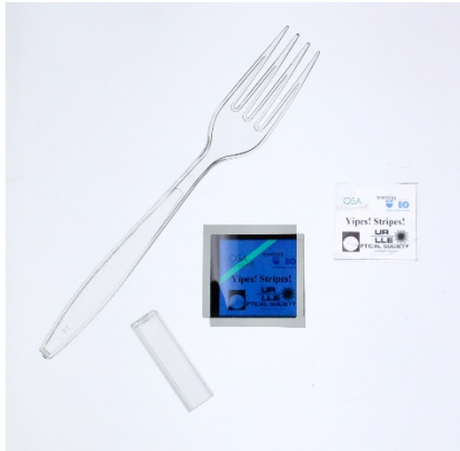
Figure 6: (a) Magic Stripes theme packet and (b) slide to show optical retardation induced by stress
