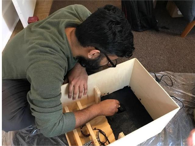
Figure 4. Unfinished color matching box and blackout painting. The unfinished color matching box (left) has tunable red, green, and blue LEDs and commercial light source mounted next to each other. A separator is placed between the sources to keep source spectra separate. To reduce the effect of wood spectral response on the light sources, the inside of the color matching box is painted black (right).
