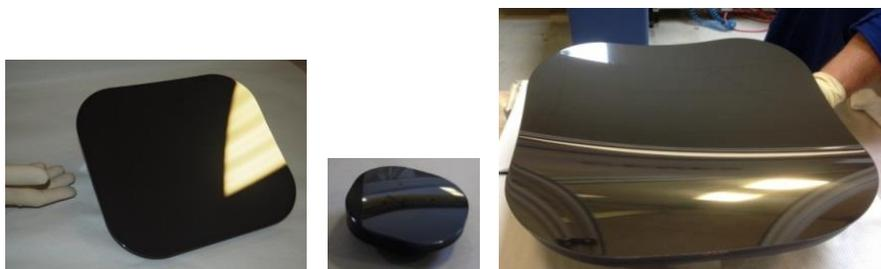
Figure 14. The IASI-NG ATA FM1 set of optics: M1 – M2 – M3 (from left to right)
