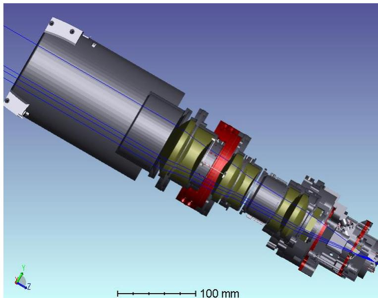
**Fig.5** : Cross-section of the non-sequential Zemax telescope model.
