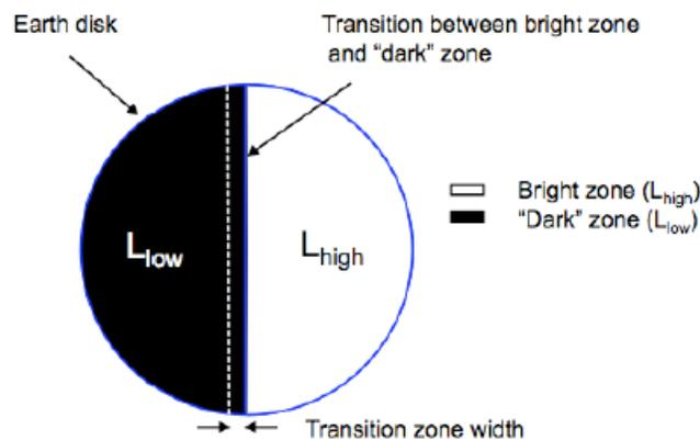
Fig.3 : Reference scene defined for S4 performance requirements.
