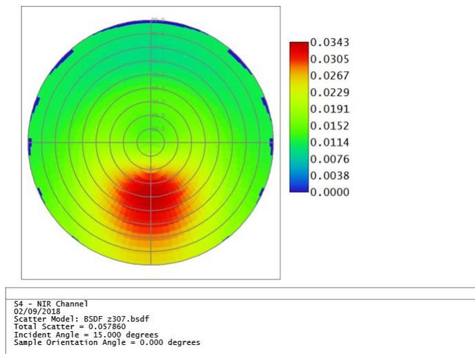
**Fig.8** : Z307 BSDF model in Zemax for angle of incidence of 15 degrees. One can see a strong forward scattering.
