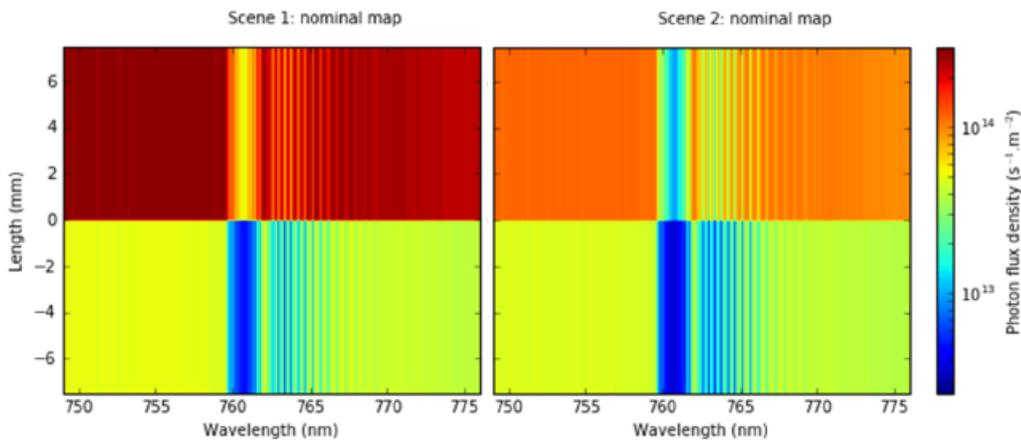
Fig.10 : Reference scenes projected on the NIR spectrometer focal plane.
