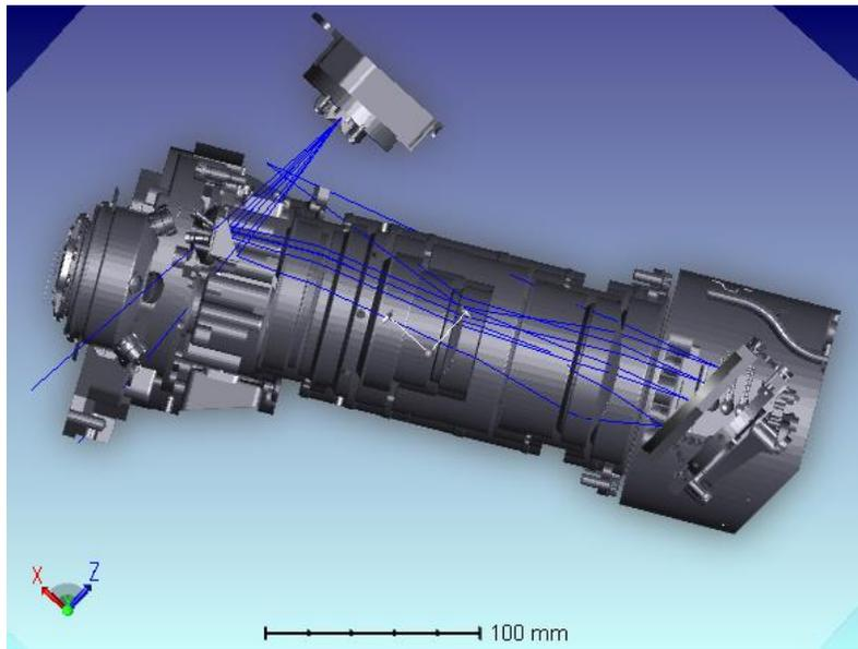
**Fig.7** : Cross-section of the non-sequential Zemax NIR spectrometer model with the slit assembly.
