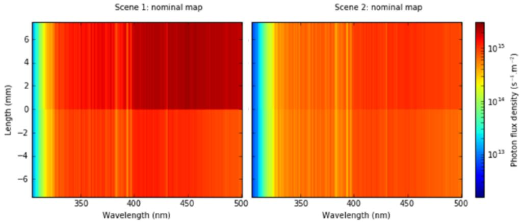
Fig.9 : Reference scenes projected on the UVVIS spectrometer focal plane.
