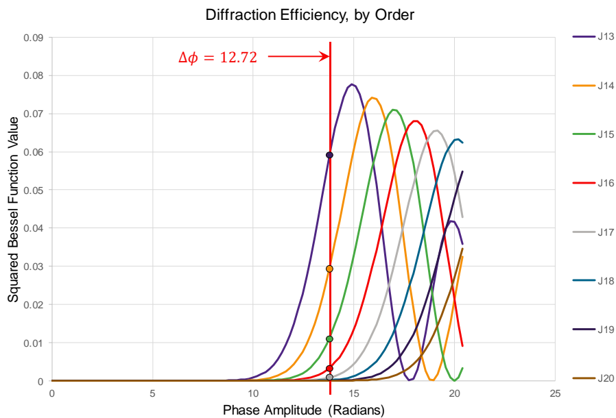
Figure 6. The Diffraction Orders outside the Snell's Law prediction.
