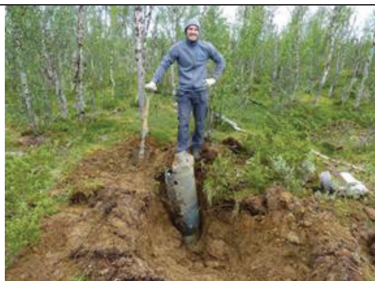
Figure 10. ROTEX-T payload after landing without parachute.
