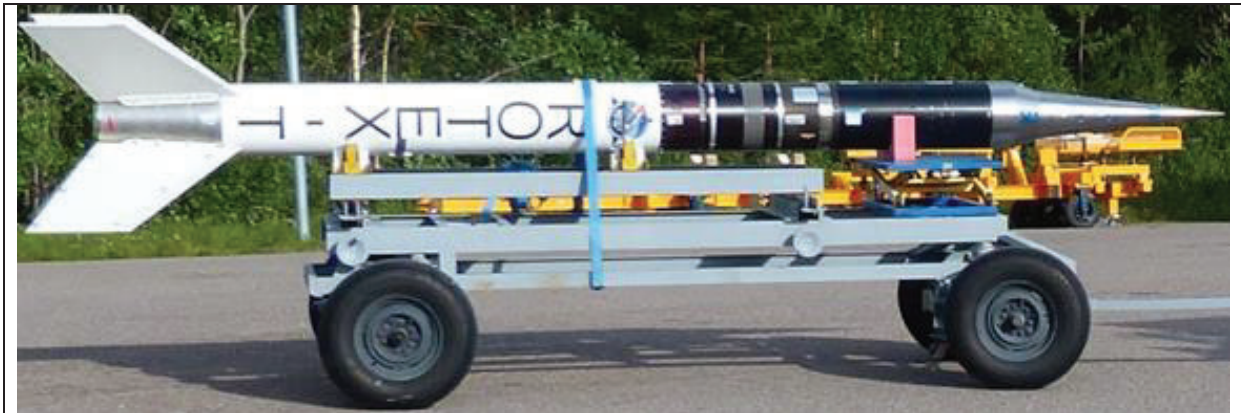
Figure 7. ROTEX-T payload mounted to second stage [10].
