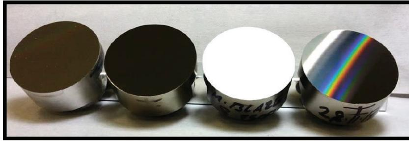
Figure 9. Freeform diffraction gratings manufactured using a 5-axis CNC machine.
