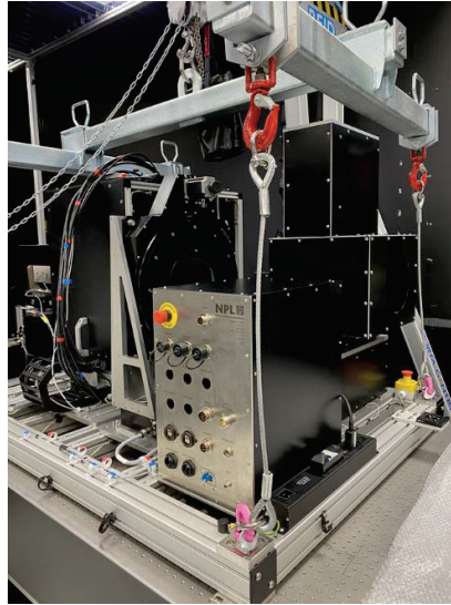
Figure 7. Picture showing a sub section of STAR being craned onto an optical table. The sub sections have repeatable interconnections for convenient re-alignment.
