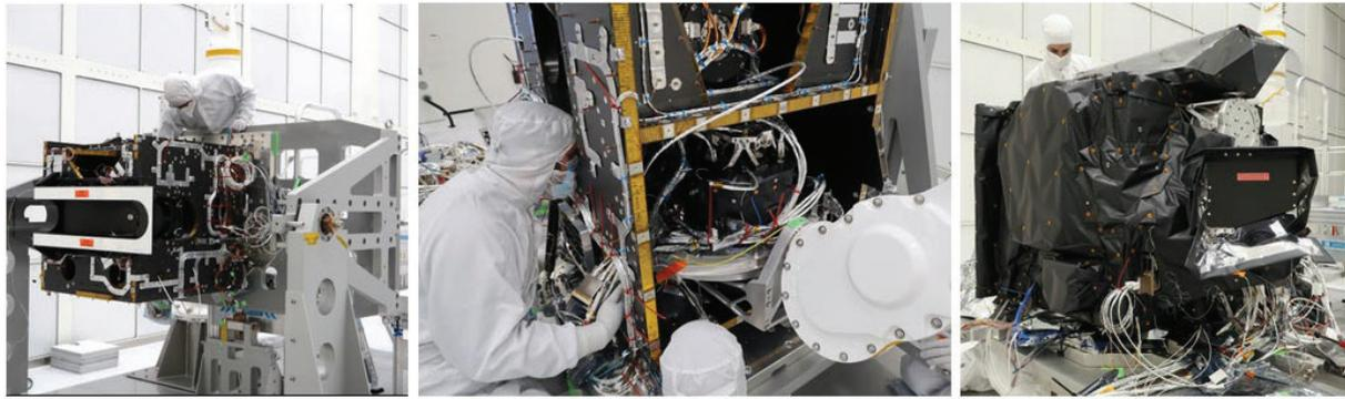
Figure 2. METimage engineering model. Integration activities on mechanical structure (left), robot supported integration of cryogenic subsystem STM into optical head (centre), and finalisation of MLI on optical head (right).
