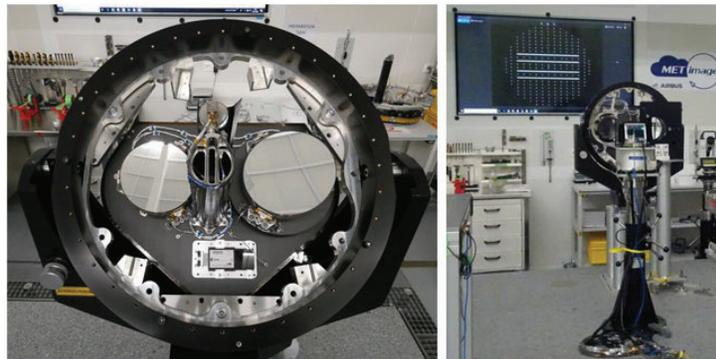
Figure 7. METimage telescope assembly first flight model (left) and telescope assembly in optical test setup (right).
