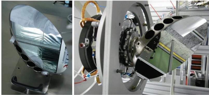
Figure 6. METimage scanner assembly first flight model. Scan mirror (left) and fully integrated scanner assembly (right).
