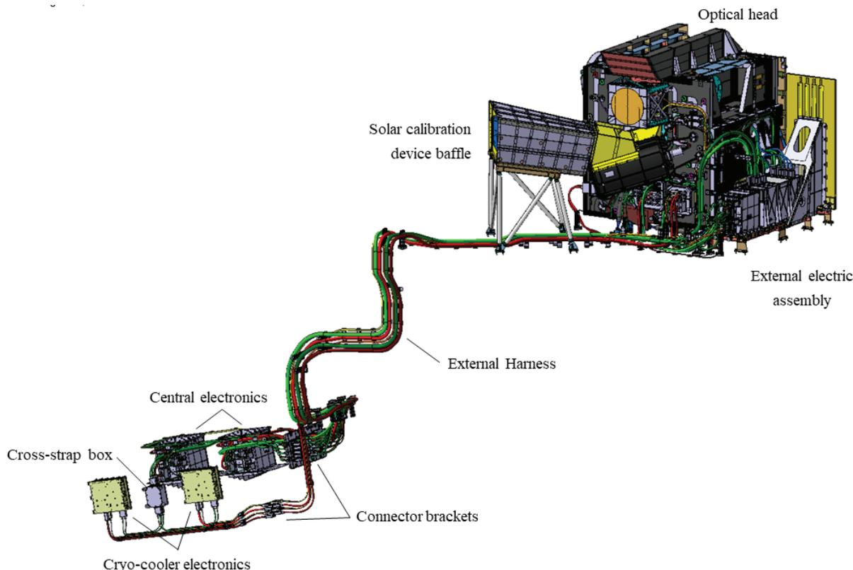
Figure 1. Overall METimage instrument configuration (MLI not shown).
