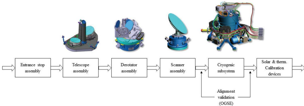
Figure 12. Integration sequence for the optical subsystems.
