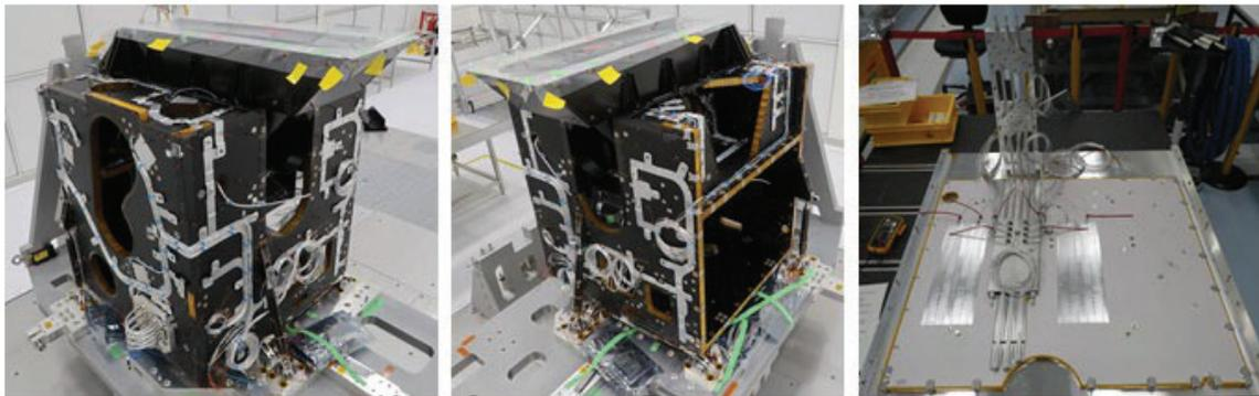
Figure 5. METimage PFM optical head thermo-mechanical assembly ready for integration of the optical subsystems.
