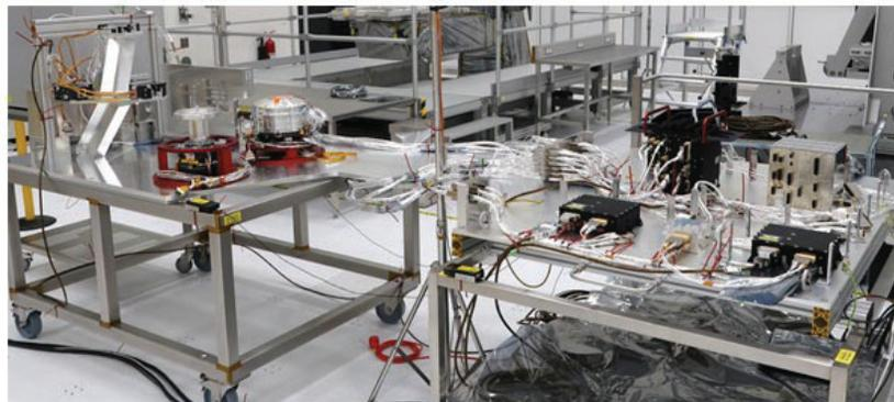
Figure 13. METimage PFM electrical-functional test bench. The electrical units of the payload equipment bay (right) and the electrical units of optical head and external electric assembly (left).
