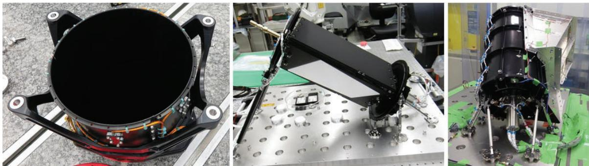
Figure 11. First flight models of the thermal calibration device (left) and of the solar calibration device (right), the latter including the Sun diffusers (centre).
