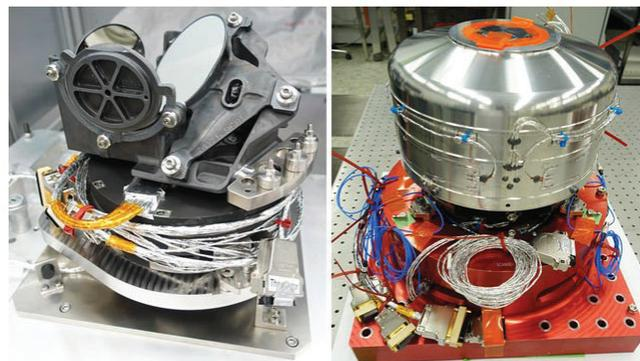
Figure 8. METimage de-rotator assembly first flight model. De-rotator optics (left) and fully integrated de-rotator assembly on vibration test adapter (right).
