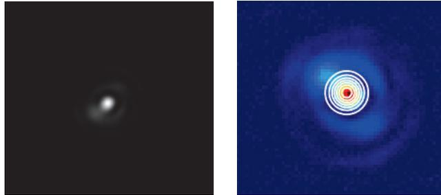
Figure 13. Receiver system PSF without turbulences in linear (left) and log (right) scale
