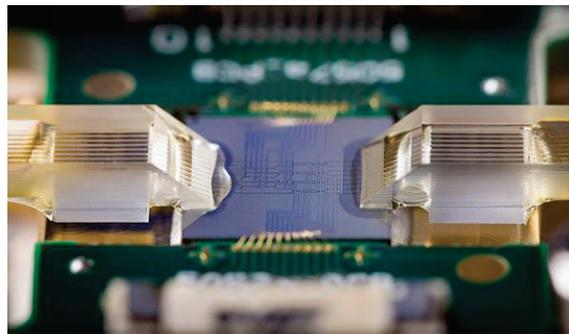
Figure 7. Close view of a photonic integrated chip (PIC) with vertical coupling through grating couplers
