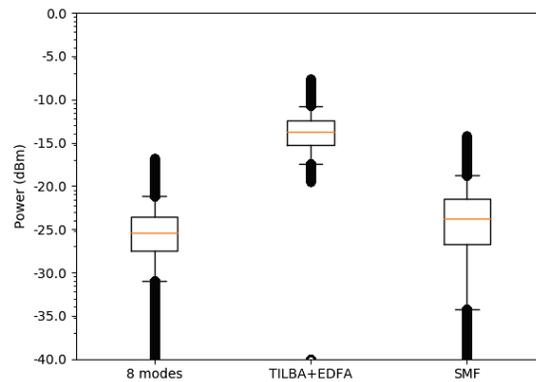
Figure 19. Statistics of collected optical power on a 1 km FSO link for an SMF, a 8-mode MPLC and a 8-mode TILBA system
