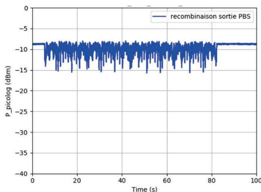
Figure 22. TILBA-ATMO output power on turbulence bench for  $D/r_0$  of 1.5 with tip-tilt compensation
