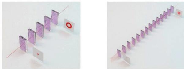
Figure 9. Multi-Plane Light Conversion principle, single-mode (left) and multi-mode (right)
