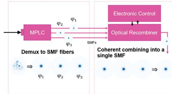
Figure 3. Turbulence mitigation scheme based on a MPLC and a coherent combining unit
