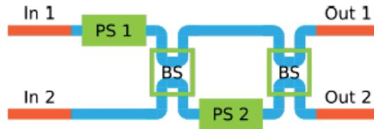
Figure 6. Two-by-two channels recombining principle using a Mach-Zehnder interferometer
