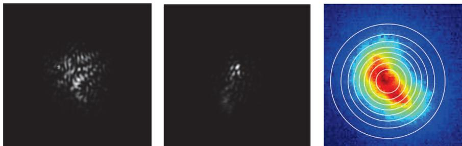
Figure 15. Instantaneous pictures of the turbulent beam (left and center) and long-time exposure (right) on the 25<sup>th</sup> of April at 2:40pm CET
