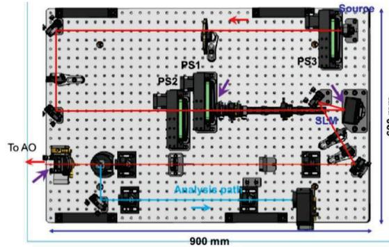
Figure 16. Schematic of the PICOLO turbulence bench at the ONERA [14]
