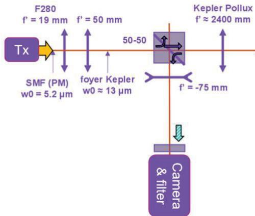
Figure 8. Schematic of the emission side of a 200 m FSO link
