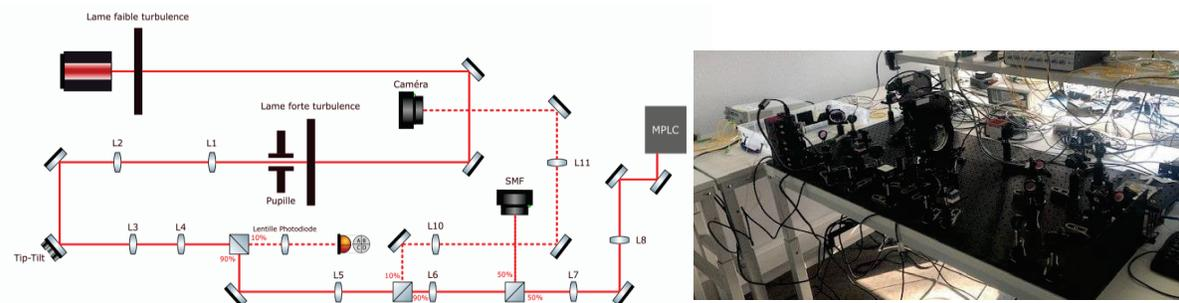
Figure 17. Cailabs' turbulence emulation bench schematic (left) and picture of it (right)
