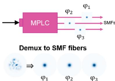
Figure 2. Demultiplexing of high orders modes into multiple TEM00 implemented by the MPLC
