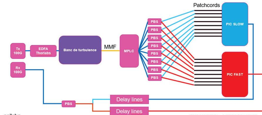
Figure 18. Schematic of turbulence mitigation experiment for a 100 G DP-QPSK telecom link
