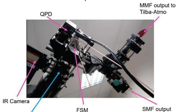
Figure 9. Receiver side of the 200 m FSO link
