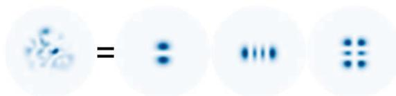
Figure 1. Example of modal decomposition of a turbulent beam
