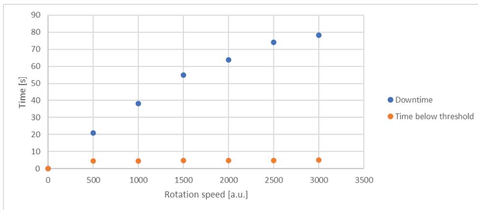
Figure 21. Evolution of link downtime and time below threshold versus phase plate rotation speed
