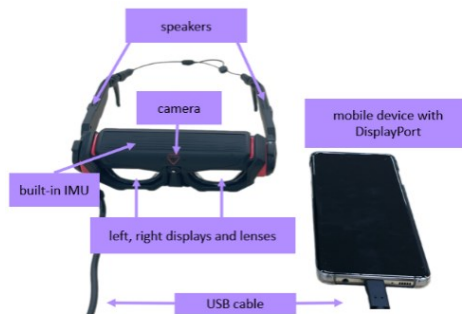
Figure 1. Optical see-through AR glasses and connection with mobile phone.
