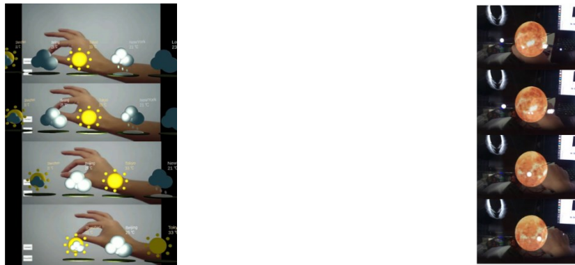
(a) Move control using a pinch gesture, sensitivity factor: 0.09 (b) Rotate control using a fist gesture, sensitivity factor: 0.0005
