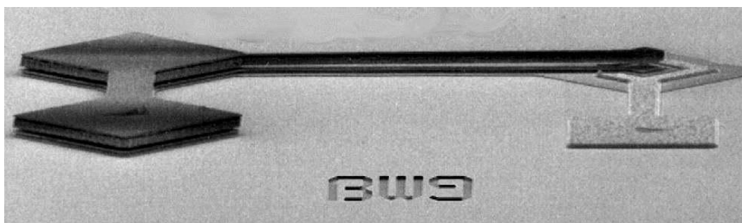
Figure 9. Tunable VCSEL with the top mirror formed by a deflectable cantilever. Courtesy Bandwidth9.
