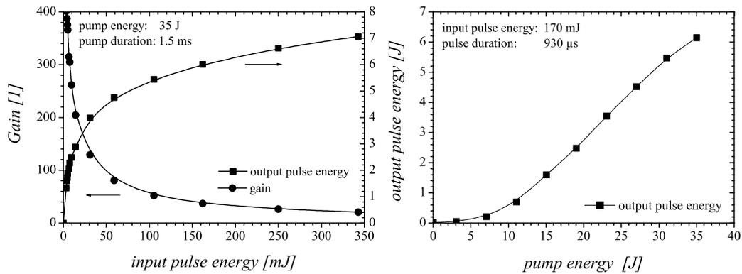
Figure 5. Millisecond pulse amplification, pulse duration:  $930 \mu\text{s}$ , numbers of passes: 4; (a) Output pulse energy and total gain vs. input pulse energy at a pump energy of 35 J, (b) Output pulse energy vs. pump pulse energy, input pulse energy: 170 mJ.
