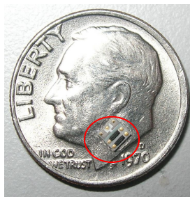
Fig. 2.3-1 (a) Mount prepared sensor on a dime.
