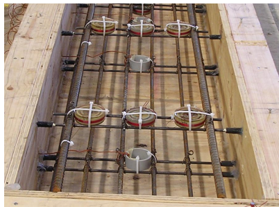
Figure 7: Top and bottom layers of reinforcement were supported independently on the transverse reinforcement in Slabs 3 and 4.
