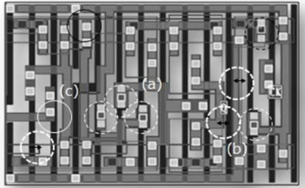
Figure 2.3.2-1. Standard cell in 45nm. (a) Double contact. (b) Recommend rule (c) Litho
