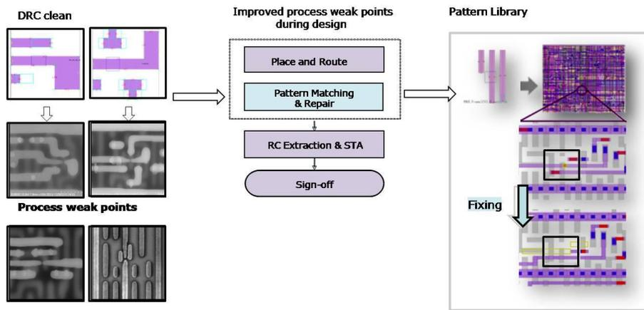
Figure 2.4.1-1. PHR (Process Hotspot Repair) flow on ECO
