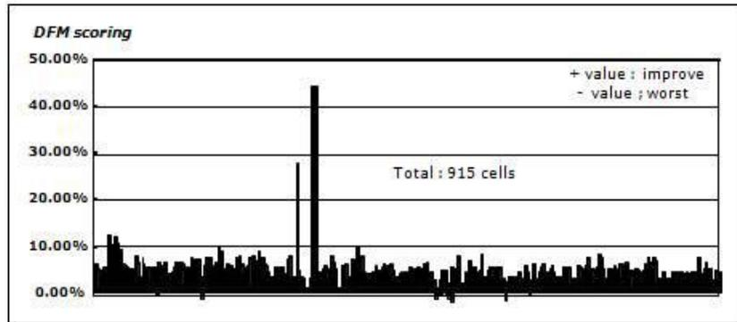
Figure 2.3.2-2. Verified results by Rule scoring after validation on 45nm standard cells
