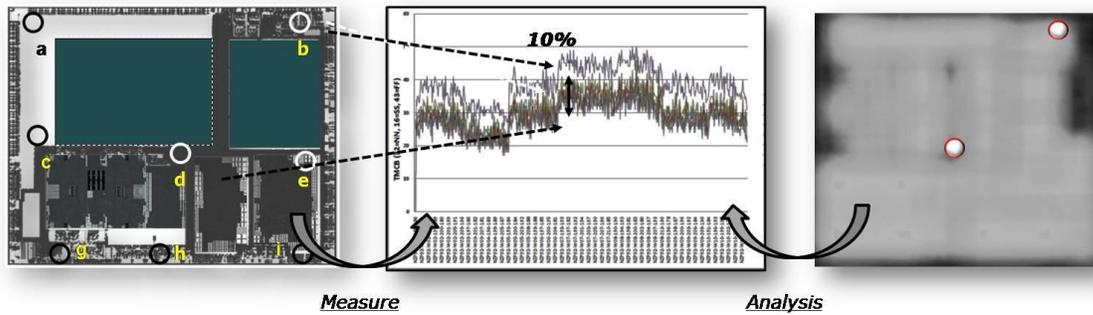
(a) Location IP for monitoring on Chip (b) Difference of center / edge Vth (c) Density map of dummy on chip
