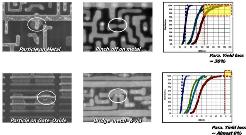
(a) Random failures (b) Systematic failures (c) Parametric failures
