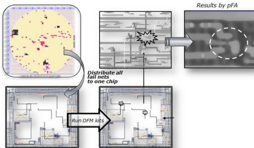
Figure 3.1.1-1. Wafer level inspection with fail nets to enable efficient pFA
