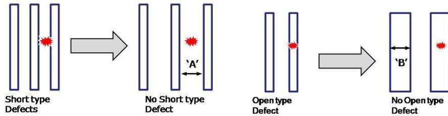
(a) Wire spreading (b) Wire widening
