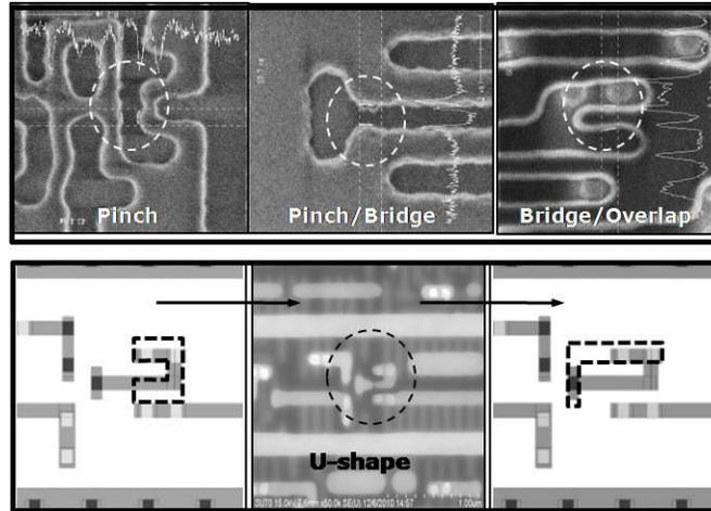
Figure 2.3.4-1. LUP (Litho Unfriendly Pattern) & status of correction for U-shape.
