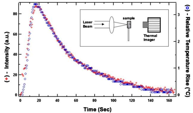
**Fig. 4** (Inset) The experimental setup for residual heat deposition measurements on bovine enamel block samples. The thermal camera was placed behind the sample to record thermal radiation from the tissue sample throughout the laser ablation. Simultaneous thermal measurements using the thermal camera (+)-left-axis and a microthermocouple (o)-right axis for 3000 laser pulses delivered with a fluence of 0.28  $\text{J}/\text{cm}^2$  and a repetition rate of 300 Hz.
