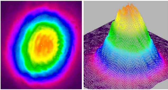
**Fig. 3** Two- and three-dimensional images of the laser spatial profile acquired using a Pyrocam III pyroelectric beam analyzer.
