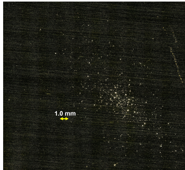
Fig. 5 Damage to the second layer of shot 6. The impactor completely disrupts after impact with the first layer, resulting in fragments that create many holes on the second membrane. A high density damage region is observed in the center, surrounded by a diffuse region of damage.
