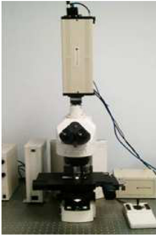
Fig. 14 Photo of the complete spectral imaging system used for the cervical cancer screening imaging.
