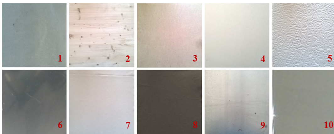
Fig. 2 The materials employed in our tests are in the order: iron, fir wood, plywood, plastic, polystyrene, reflective surface, white fabric, dark fabric, aluminum, and glass.
