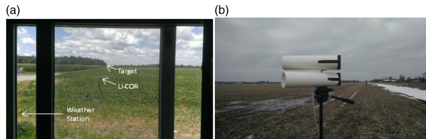
Fig. 7 (a) View from Harris farm test site trailer window, and (b) simulated plume setup to test 2-D reconstructions by subjecting specific chords to CO 2 enhancement.
