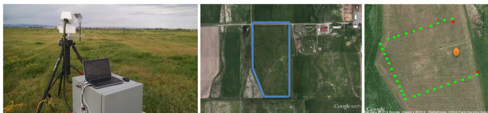
Fig. 8 Initial GreenLITE system testing at the ZERT facility in Bozeman, Montana. Orange dot indicates where the in situ instrument was placed for the comparisons in Sec. 4.
