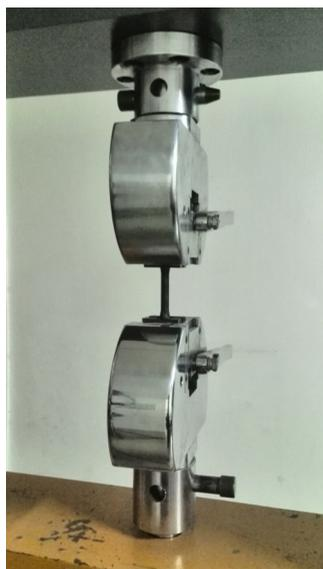
**Fig. 3** The tensile test at room temperature of speckled and un-speckled specimens.
