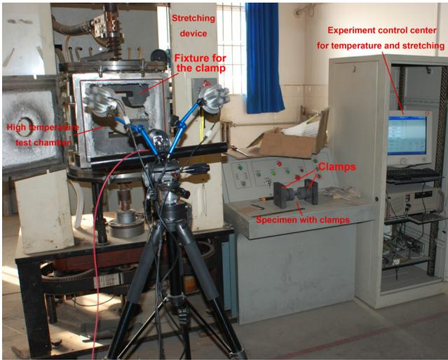
Fig. 22 Heating and stretching devices.
