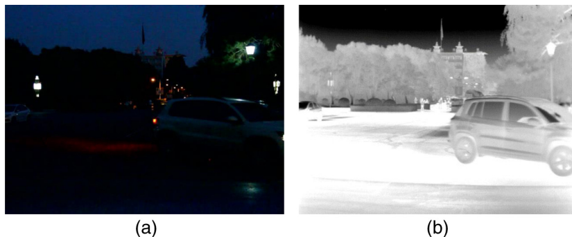
Fig. 4 Original images: (a) original low-light visible image and (b) original infrared image.
