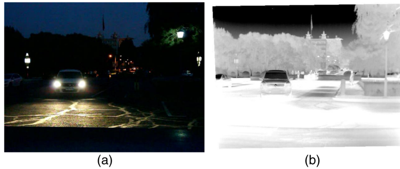
Fig. 6 Original images: (a) original low-light visible image and (b) original infrared image.
