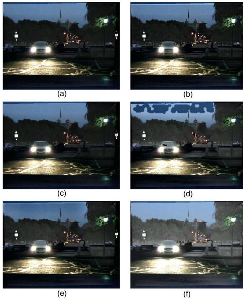
Fig. 7 Fused color image: (a) WT with two levels, (b) WT with four levels, (c) traditional contourlet transform, (d) OI-PCNN algorithm, (e) GFF algorithm, and (f) proposed method.
