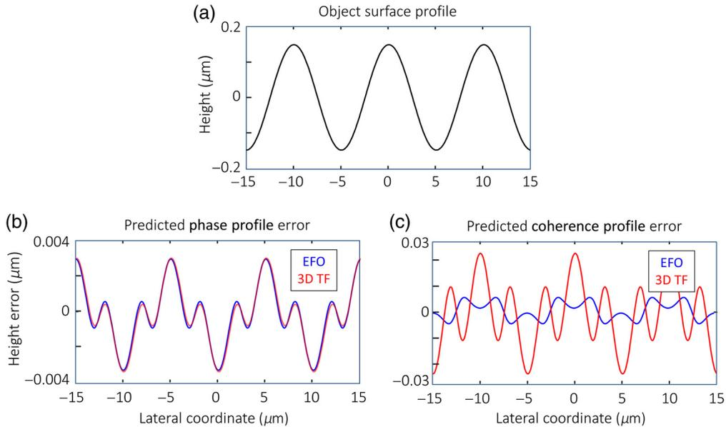
**Fig. 15** (a) Simulations for the EFO and 3D TF models at  $\text{NA} = 0.55$  (50 $\times$  objective) for a sinusoidal profile with an amplitude of  $0.15 \mu\text{m}$ . The mean wavelength is  $0.57 \mu\text{m}$  and the FWHM bandwidth is  $0.08 \mu\text{m}$ . The predicted measurement errors for (b) the phase profile and (c) the coherence profile.
