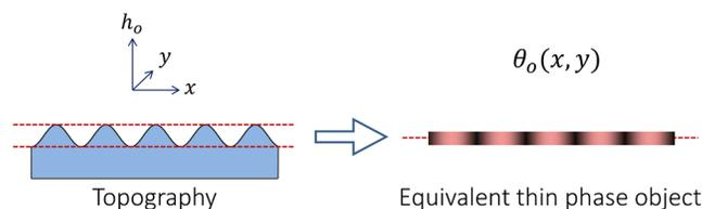
**Fig. 5** The thin phase object approximation, assuming that the topography variations are small relative to the DOF. The color density in the equivalent thin object represents phase variations of a complex amplitude reflectivity.
