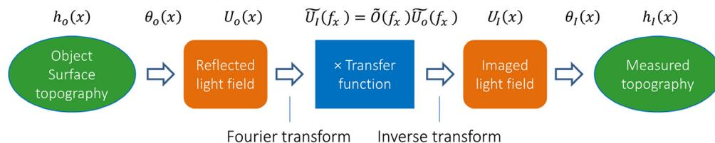
**Fig. 7** The EFO model for a single wavelength.
