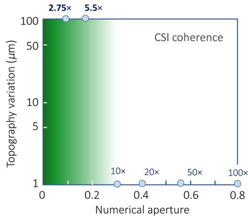
**Fig. 13** Limits to applicability of the EFO model for CSI for coherence profiles using common light sources. The white light approximation is limited to low NA values characteristic of objective magnifications below 10 $\times$ .
