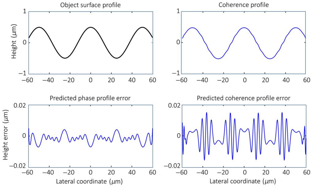
**Fig. 8** Simulated measurement results using the EFO model for the profile of Fig. 1. The sinusoidal period is  $50 \mu\text{m}$ , and the peak-valley height range is  $1 \mu\text{m}$ . The mean wavelength is  $0.5 \mu\text{m}$ , the FWHM bandwidth is  $0.1 \mu\text{m}$ , and the NA is 0.1.
