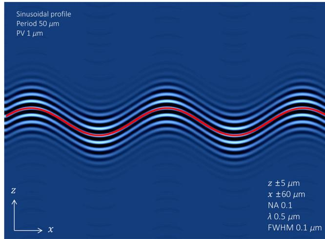
**Fig. 1** Simulated interference signal detected by a camera for a sinusoidal surface topography when using a spectrally broadband light source, as the interference objective is scanned in the  $z$  direction. The central red line represents the object surface profile on the same scale.
