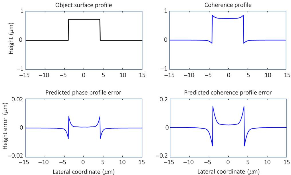
**Fig. 9** Simulated results using the EFO model for an  $8\text{-}\mu\text{m}$  wide rectangular surface feature with a height of  $0.75 \mu\text{m}$ . The mean wavelength is  $0.57 \mu\text{m}$ , the FWHM bandwidth is  $0.12 \mu\text{m}$ , and the NA is 0.15. Note the  $10\times$  difference in height scale for the predicted errors for the coherence and phase profiles.
