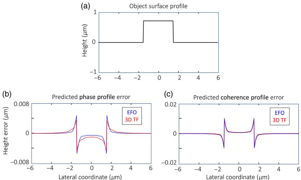
**Fig. 16** (a) Simulations for the EFO and 3D TF models  $\text{NA} = 0.55$  (50 $\times$  objective), for a rectangular profile similar to that shown in Fig. 9, with a width of  $3 \mu\text{m}$  and a height of  $0.75 \mu\text{m}$ . The mean wavelength is  $0.57 \mu\text{m}$  and the bandwidth is  $0.14 \mu\text{m}$ . The predicted measurement errors for (b) the phase profile and (b) the coherence profile.
