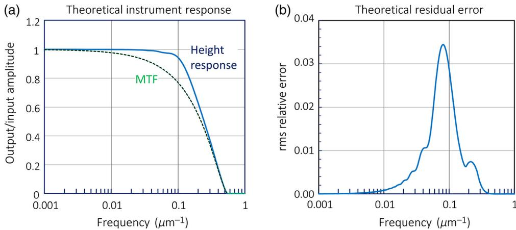
**Fig. 10** EFO modeling analysis of instrument response as a function of surface spatial frequency for phase profiles, for a constant maximum surface slope equal to 50% of the geometrical NA limit. (a) The results in comparison with the optical imaging MTF and (b) the rms error in the measured profile. The mean wavelength is  $0.57 \mu\text{m}$  and the NA is 0.15.
