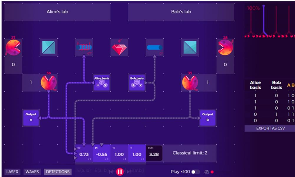
**Fig. 11** An experimental setup for the CHSH Bell Inequality violation. Note that the experiment depends on two random variables (Alice's and Bob's basis), provides a table of all measurements (downloadable as a CSV file), and presents all correlation in real time.
