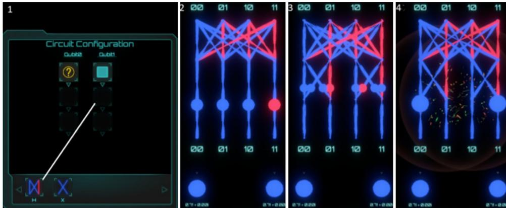
**Fig. 13** Images 2, 3, and 4 are snapshots of the evolution of a quantum state vector in visual form for two particles that start in the ground state 00 and reach the Bell state 00 and 11. The balls at the bottom show the desired output solution, and the user is required to place a Hadamard gate to achieve it as shown in 1.
