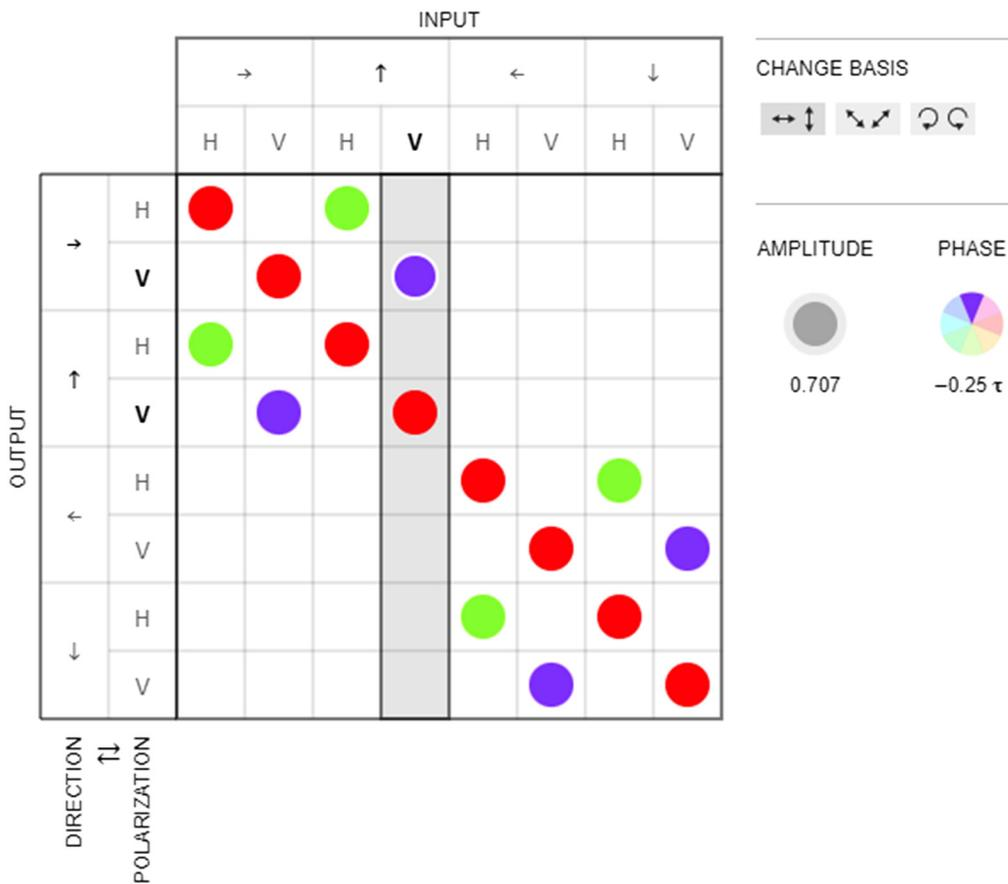
**Fig. 12** A matrix visualization for a beamsplitter with BraKetVue. The matrix values are presented with a circle size (radius for the amplitude, area for the probability) and color (hue for the phase). Index labels incorporate the tensor structure.
