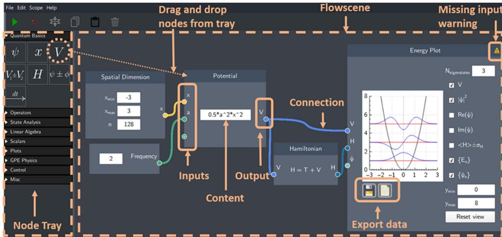
**Fig. 16** The Quantum Composer interface. Users can drag-and-drop nodes (representing space, the potential, a plot, etc.) from the left-hand tray into the simulation space (called a flowscene). Connections are then made between the nodes to direct information from one node to another. This figure shows how one can set up a simulation that shows the first three eigenenergies and eigenstates of the quantum harmonic oscillator. Figure reproduced from Ref. 87.
