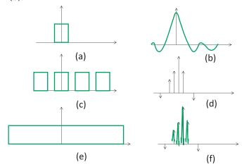
**Infinite periodic series**: If a **periodic signal**, as shown in (c), is created by repeating the pulse, this case is equivalent to convolving with a series of impulse functions (remember that in sampling, it was a multiplication). The frequency domain will be modified by a multiplication with the spectrum of this impulse series.
