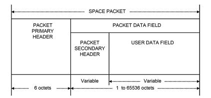
Figure 5.1 Space packet structural components (image courtesy of CCSDS).
