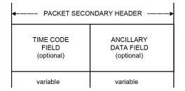
Figure 5.3 Space-packet secondary header (image courtesy of CCSDS).
